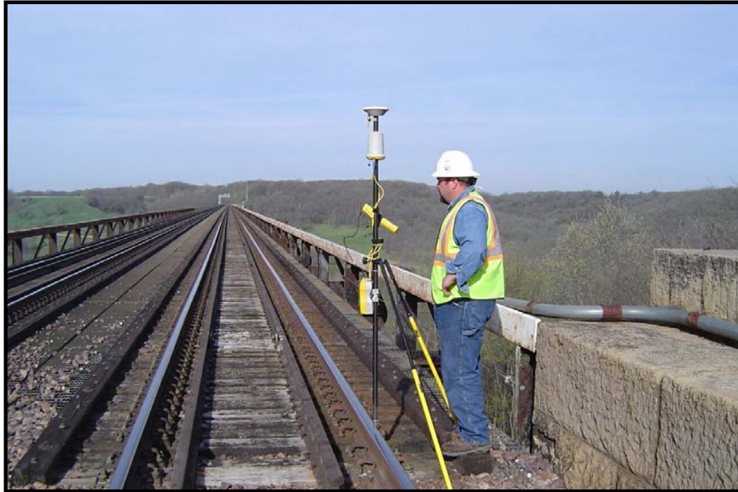
Steve Lentz, WHKS survey technician, observing a GPS point for an Iowa survey project.
